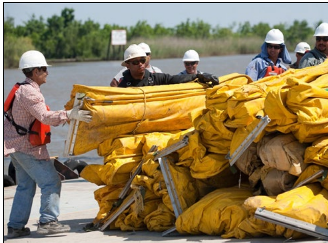
United States Environmental Services workers prepare oil containment booms for deployment Source: Wikipedia
